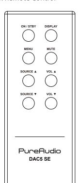
ON / STBY: Press to put the unit into standby mode or turn it on.
