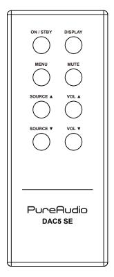
ON / STBY : Press to put the unit into standby mode or turn it on.
